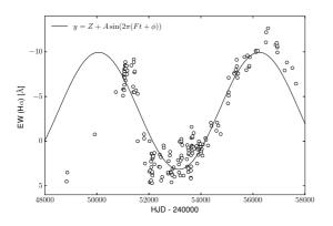
**Fig. 4.** The Least-Squares Fit for data gained by Period04. Z = -3.39 as the zero point, A = 6.56 Å as the amplitude,  $F = 0.000162 d^{-1}$  as the frequency,  $\phi = 0.639$  as the phase and t as the time.
